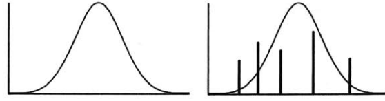
Figure 5-3: (left) A normal distribution H \sim N(\mu, \sigma^2) and (right) G \sim DP(H, \alpha) , with H interposed for reference. G is a probability distribution that “looks like” H , but whose distribution is discrete.
